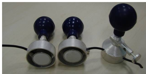
Fig. 2 Vacuum electrodes for acquiring heart sound signal and ECG simultaneously
